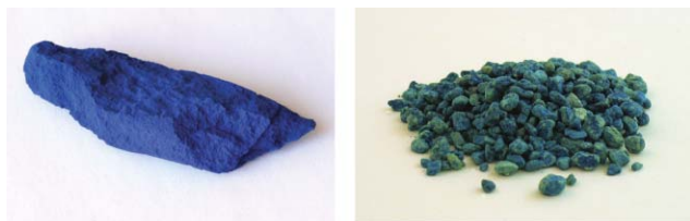
Fig. 2 A piece of industrially produced Ultramarine Blue (left) and Maya Blue produced from sepiolite (right). The sepiolite stems from commercially available cat litter.
