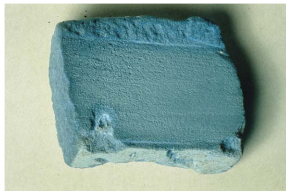
Fig. 14 Brick Nimrud. A Mesopotamian building block made from Egyptian Blue and quartz, presumably along the lines of the “compact body procedure” (see text). © Copyright the Trustees of The British Museum.
